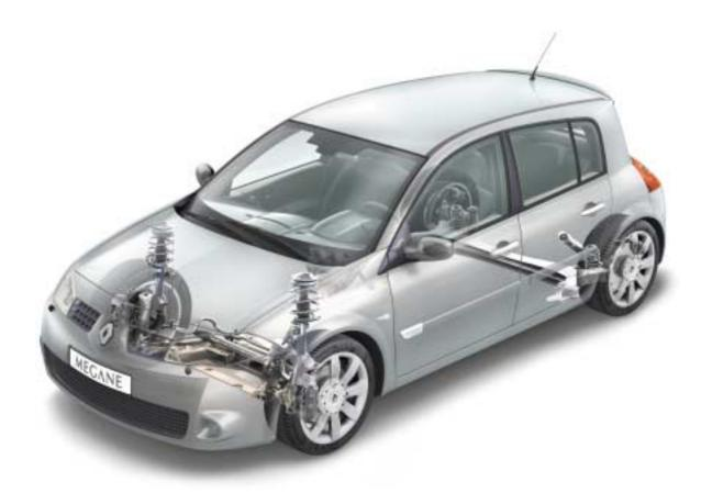
The Mégane Renault Sport carries over the platform design of Mégane II with its wheelbase of 2,625mm. Its front and rear tracks have been increased to 1,517mm (+ 7mm) and 1,521mm (+ 15 mm) respectively to the benefit of stability and grip.
