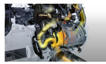
A 1,598-cm<sup>3</sup> engine delivering 130 hp, the **Energy dCi 130** is the most powerful diesel engine in its category. Generous torque, a full 80% of which is available from just 1,500 rpm and across a broad operating range, brings drivers lively pick-up for an immensely enjoyable at-the-wheel experience. With considerable reach for a diesel engine, the Energy dCi 130 revs up easily to 4,500 rpm, providing the driving pleasure of a
