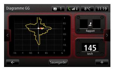
For even more fun, users can display a G-force diagram to measure longitudinal and lateral acceleration and save the highest values. The wheel spin of driven wheels is also available.
