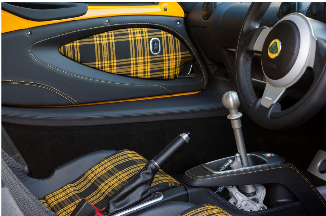
The Lotus Exige Sport 350 is also available with a 6-speed automatic option where drivers can change gears manually via forged aluminium paddles located behind the steering wheel, or rely on the gearbox's fully automatic mode. The automatic gearbox control panel is integrated neatly into the centre console of the cockpit, with buttons for Park, Reverse, Neutral and Drive. Up-shifts take just 240 milliseconds, with rapid downshifts accompanied by automatic throttle-blip (when in Sport mode).
