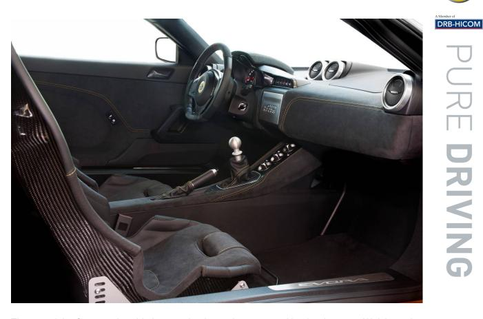
The rest of the Sport 410's cabin has received attention as part of its development. Weight saving measures includes attractive one-piece door trim panels finished in Alcantara®, with contrast stitching, the deletion of door arm rests and stowage pockets, the relocation of tailgate and fuel filler release buttons and the removal of speakers - if an entertainment system is not specified.
