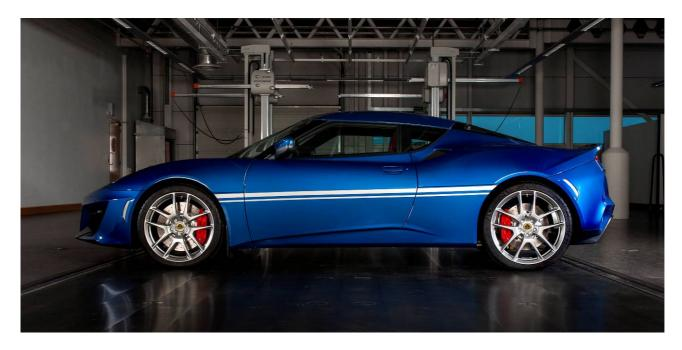
Over two thirds of the Lotus Evora 400 has been revised, including its supercharged and charge-cooled, mid-mounted, 3.5-litre V6 engine, which produces 400 hp and 410 Nm of torque. This complements a revised aluminium chassis, which offers increased torsional rigidity and reduced weight.
