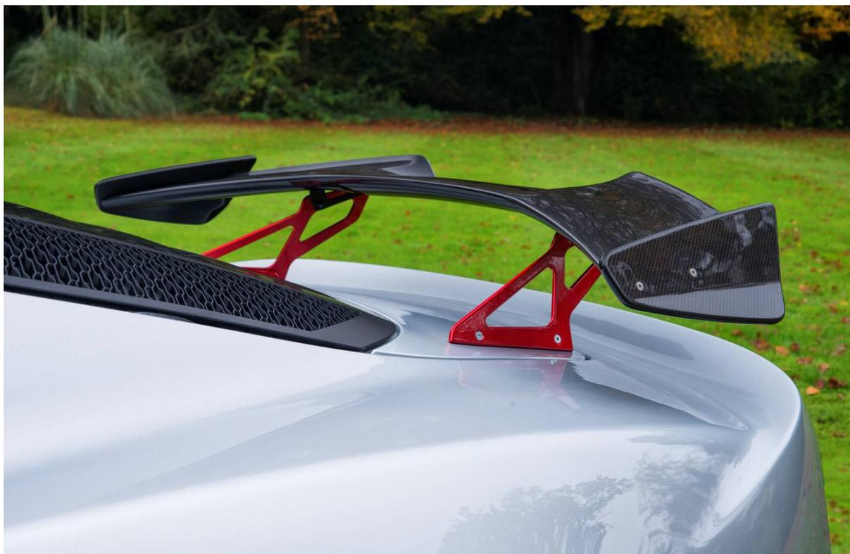
In addition, twin pairs of front canard wings, mounted forward of the front wheels, a carbon rear wing and air blades behind the rear wheels, all work to help raise downforce to a massive 140 kg at maximum speed - a 60% gain over the Exige Sport 350, which generates 88 kg at its maximum
