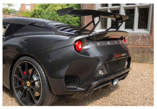
To harness the increased downforce and power, mechanical grip is provided by 10 mm wider Michelin Pilot Sport Cup 2 tyres, with 245/35 R19 at the front and 295/30 R20 at the rear, on one inch wider 10.5J rear wheels. Ultra-lightweight forged aluminium wheels are standard, in either black or silver, with optional finishes available in gloss red or a gloss black machined rim design.
