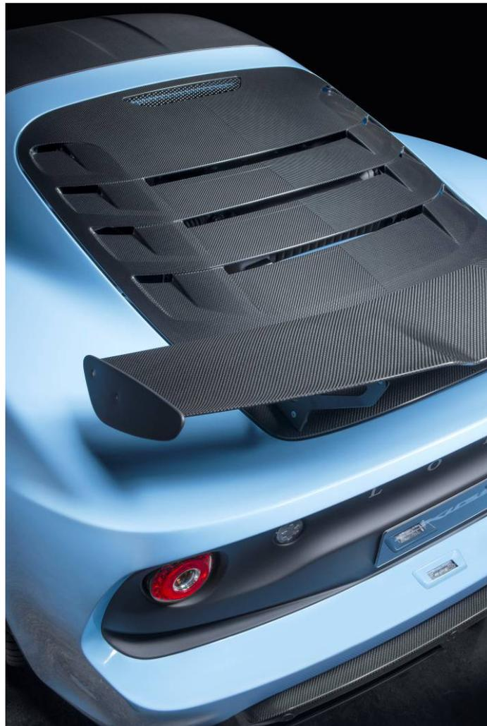
Distinctive in its appearance, thanks to wider aperture grilles in the new front clam panel, the Exige Sport 410's revised aero configuration provides total downforce of 150 kg (60 kg at the front and 90 kg at the rear); developed through extensive CFD modelling and wind tunnel testing in order to preserve the car's handling balance and high-speed stability.
